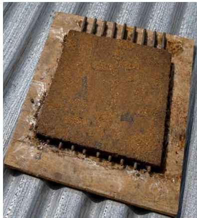
Gambar 22 Penjemuran Sadake Board Lubang 9
