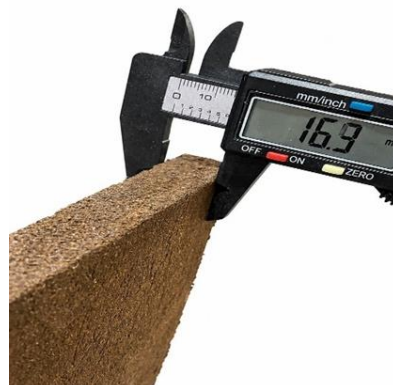
Gambar 24 Pengukuran Ketebalan Sadake Board
