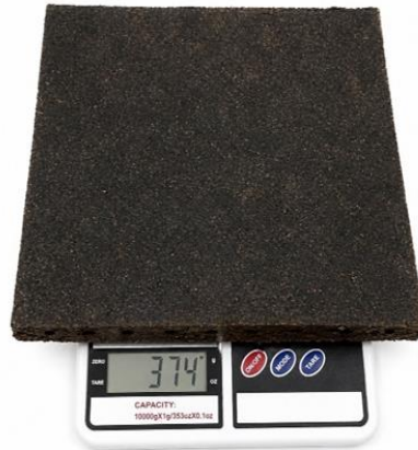
Gambar 25 Pengukuran Massa Sadake Board
