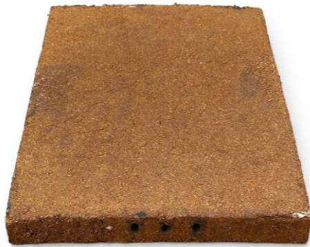
Gambar 15 Sadake Board (fiberboard) Lubang 3
