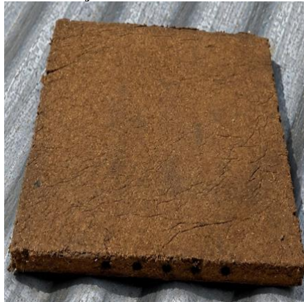
Gambar 20 Penjemuran Sadake Board Lubang 5
