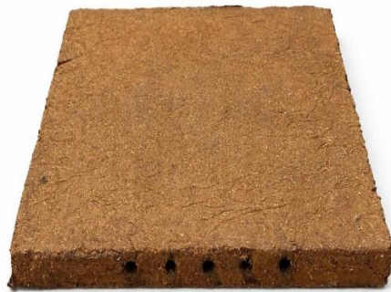
Gambar 16 Sadake Board (fiberboard) Lubang 5
