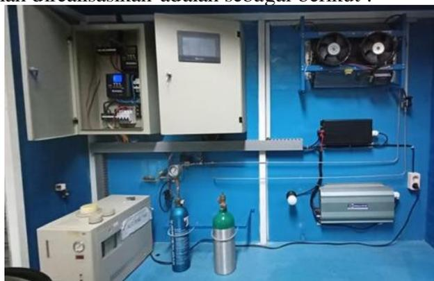
Gambar 5. prototype Stasiun Pengisian Gas Hidrogen (Refuelling Hydrogen Gas Station)
