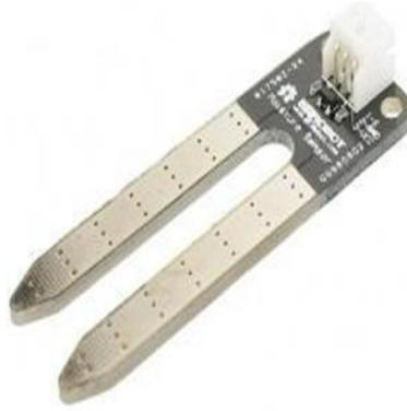
Gambar: Sensor Kelembaban Tanah
