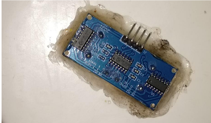
Gambar 3 Rangkaian Sensor Ultrasonic
