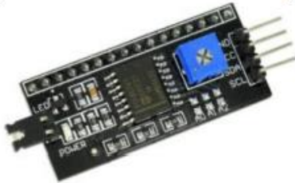
Gambar 7 Modul I2C LCD
