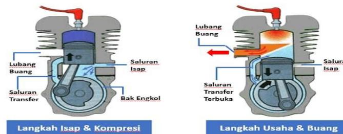
Gambar 2 *Diesel Engine 2 Stroke*
